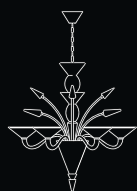
L 75 8+3 LUCI/LIGHTS Ø 98 - H 100 cm 8 E14 max 60W + 3 LED G4 max 1,5W 15 Kg
